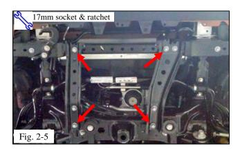
(f) Use a 17mm hex socket to remove the four bolts (M12 x 1.25 x 28mm) from the member braces (Fig. 2-5).
