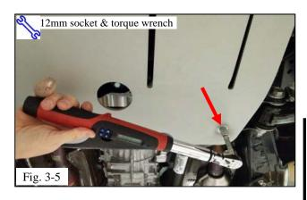
(i) Torque the rear bolts to 29 N-m (21 ft-lbf) (C, Fig. 3-3 and Fig. 3-5).
