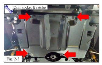
(d) Use a 12mm socket to remove the four bolts (M8 x 1.25 x 20mm) that secure the front skid plate (Fig. 2-3).
