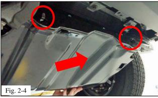
(e) Push the skid plate forward to release it from the two hooks (circled) on the forward edge (Fig. 2-4).
